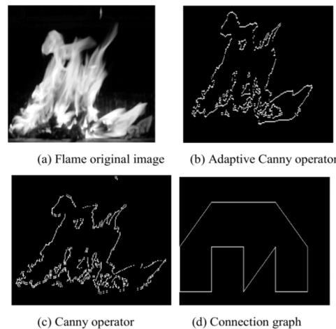
Fig. 3. Steps of Canny Edge Detection [1]
