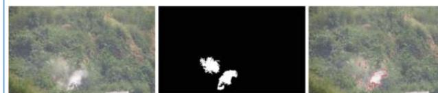
Fig. 6. Original Image (Left), 3DFCN Isolation of the Smoke After Detection (Middle), Smoke Outlined Based on the Isolated Image (Right). [4]
