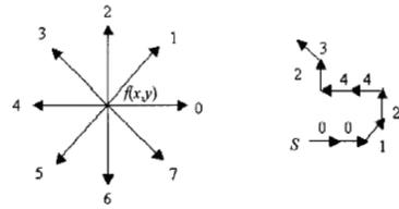
Fig. 2. Potential Gradients Adjacent to a Pixel (LEFT). Edge Tracing Using Sharpest Gradients (Right) [1]
